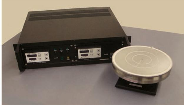
*AC controller is designed to minimize noise spikes, shown with Thermal Chuck.*
